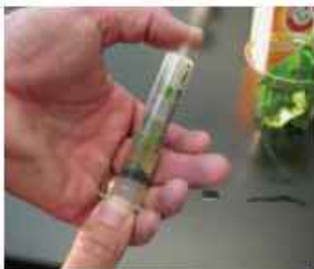
Figure 6a. Creating a Vacuum in the Plunger
